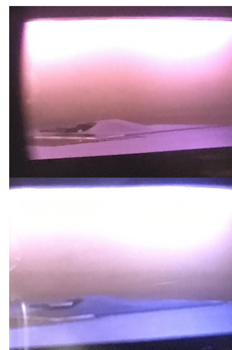
The top is an image of our sputter gun striking a primarily argon plasma with DC. The image below it is the same sputter gun combined with the HiPIMS signal. The blueness is an effect of the increased degree of self sputtering of the carbon target.
